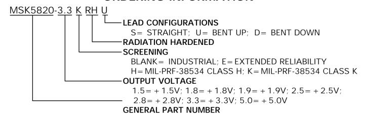
The above example is a +3.3V, Class K regulator with leads bent up. NOTE: See DSCC SMD 5962F09216 for DSCC part number options.
