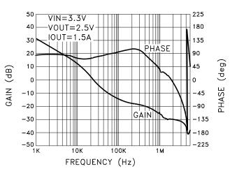
MSK5820-2.5RH GAIN AND PHASE vs. FREQUENCY
