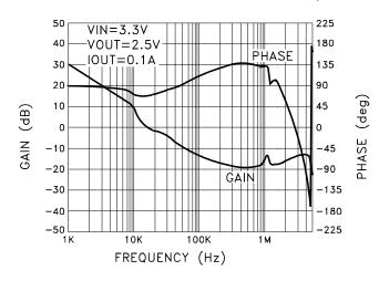
MSK5820-2.5RH GAIN AND PHASE vs. FREQUENCY
