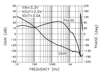
MSK5820-2.5RH GAIN AND PHASE vs. FREQUENCY
