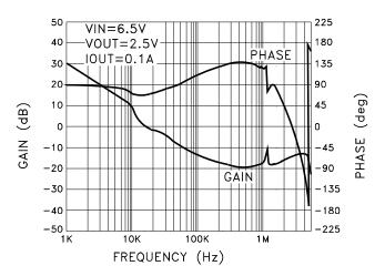
MSK5820-2.5RH GAIN AND PHASE vs. FREQUENCY
