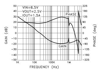
MSK5820-2.5RH GAIN AND PHASE vs. FREQUENCY
