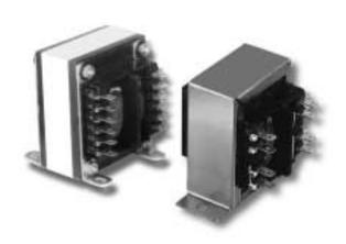
The RL-2261 Series International Power Transformers are manufactured to meet UL, CSA, VDE and IEC specifications. These transformers with chasis mount capability are available in ratings of 25VA, 43VA and 80VA. Designed with dual primaries (115/230V - 50/60Hz) and input range of (100V to 130V or 200V to 260V - 50/60Hz) and triple outputs (5VDC with ±12VDC or 5VDC with ±15VDC). The split bobbin construction eliminates the need for electrostatic shielding. HIPOT tested at 4000VRMS.
