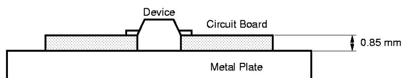
**2. Mount Pad on a Circuit Board and Soldering Area on a Metal Plate**
