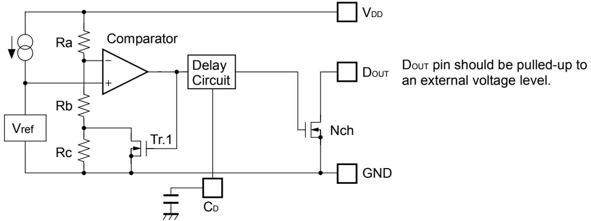
Block Diagram of External Capacitor Connection
