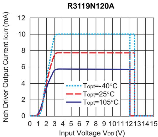
5) Nch Driver Output Current vs.  $V_{DS}$
