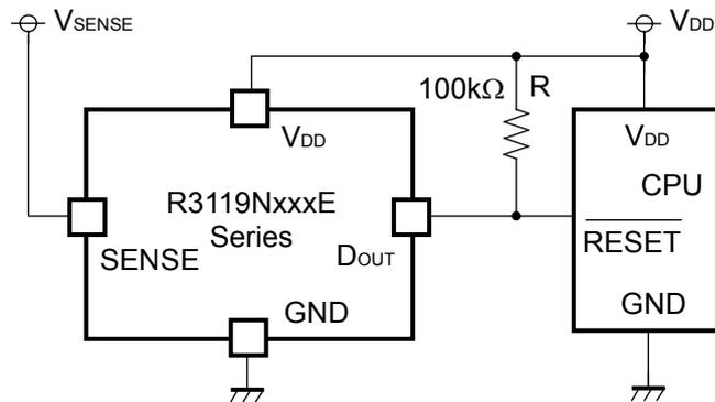
(2) Input Voltage to R3119NxxxE is unequal to Input Voltage to CPU
