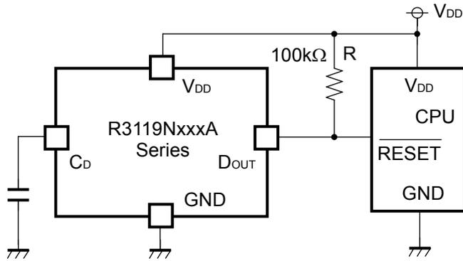
(2) Input Voltage to R3119NxxxA is unequal to Input Voltage to CPU
