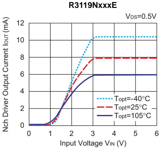
13) Nch Driver Output Current vs.  $V_{DS}$
