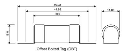
The range of Joint Service Fuse Links was originally developted for the Admiralty, but is now classified under the N.A.T.O. Reference system, Ref. Number 5920.99 The fuse links have been type approved and include short circuit tests to BS88, at 440 volts 33kA.
