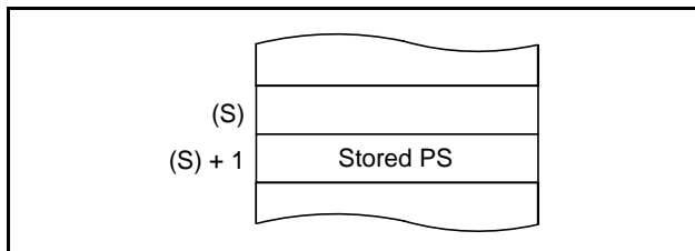
Fig. 102 Stack memory contents after PHP instruction execution
