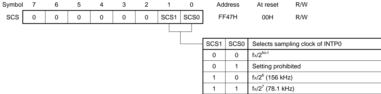
Figure 5-8. Format of Sampling Clock Select Register ( \mu PD78014, 78014Y, 78018F, 78018FY, 78014H subseries)
