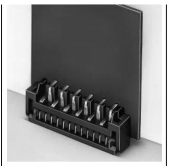
Thanks to the hinged connection of the connector, the boards can be rotated 90° so that they can be moved from parallel to vertical positions even when electricity is turned on. Thus circuit checks and adjustment of the equipment is possible even in tight spaces. Header leads are staggered for vibration resistance and for easy board design.
