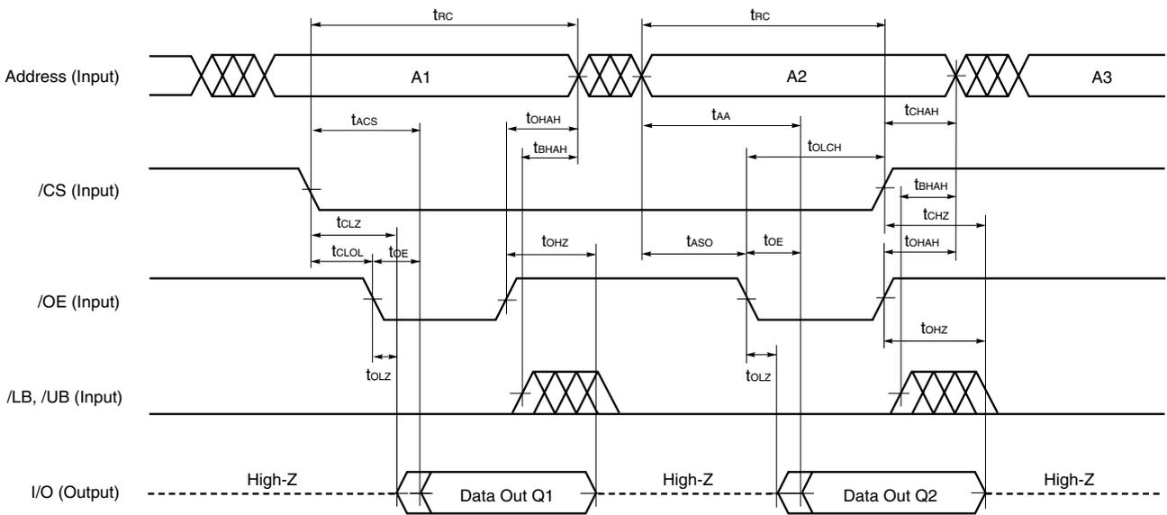
**Remark** In read cycle, MODE and /WE should be fixed to high level.
