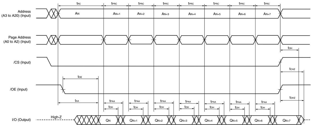
**Remarks 1.** In read cycle, MODE and /WE should be fixed to high level.
