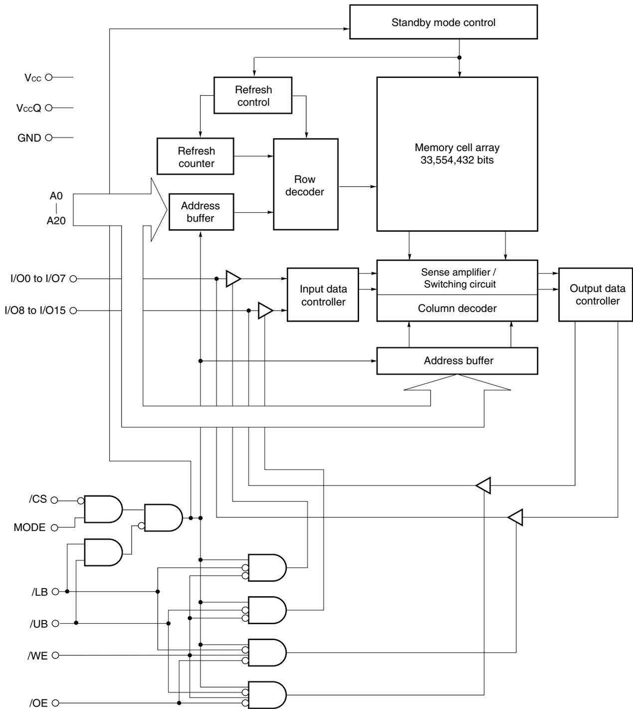
**Remark**  $V_{ccQ}$  is the input / output power supply for -BE75X and -BE85X.
