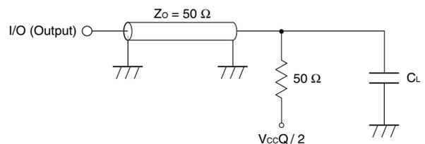
Remark C<sub>L</sub> includes capacitance of the probe and jig, and stray capacitance.
