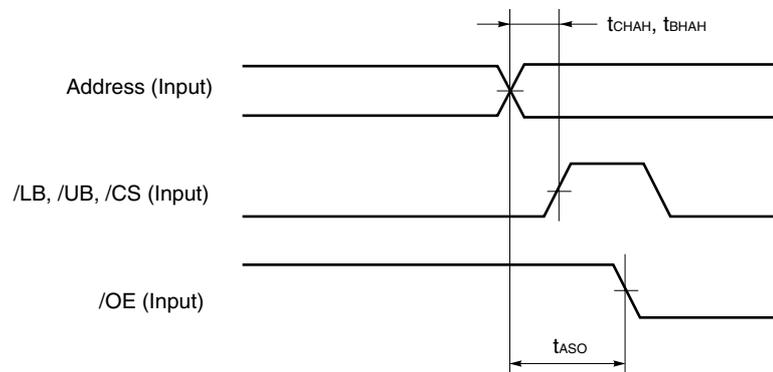
4. t<sub>BH AH</sub> is specified from when both /LB and /UB become high level.
