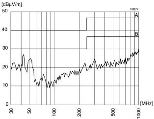
Fig. 20 Typical radiated electromagnetic field strength (quasipeak) according to CISPR 11/22 and EN 55011/22, normalized to a distance of 10 m, measured at U<sub>i nom</sub> and
