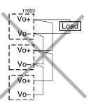
Fig. 27 An example of poor wiring for connection in parallel
