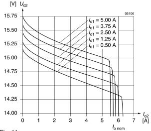
Fig. 11 AK...EK 2540:  $\Delta U_{o2}$  (typ.) vs.  $I_{o2}$  with different  $I_{01}$
