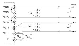
Fig. 17e AK...EK 2000 with H15 connector. R-input for output voltage control. Wiring of main and second output for two output voltages  $U_{01}$  and  $U_{02}$ : 12 V/12 V or 15 V/15 V or 24 V/24 V, the outputs are galvanically isolated.
