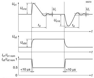
Fig. 8 Typical dynamic load regulation of  $U_{o1}$  and  $U_{o2}$
