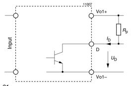
Fig. 31 Option D5…DD: NPN output, U<sub>o1</sub> ≤ 40 V, I<sub>D</sub> ≤ 20 mA
