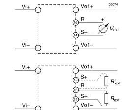
Fig. 16 Output voltage control for single output units AK...EK 1000 by means of the R input
