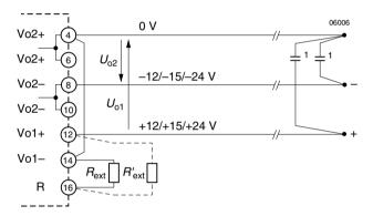
Fig. 17c AK...EK 2000 with H15 connector. R-input for output voltage control. Wiring of main and second output for two symmetrical output voltages  $U_{01}$  and  $U_{02}$ :  $\pm 12~V$  or  $\pm 15~V$  or  $\pm 24~V$ .
