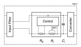
Fig. 25 Option E block diagram
