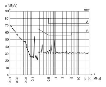
Fig. 19 Typical disturbance voltage (quasi-peak) at the input according to CISPR 11/22 and EN 55011/22, measured at  $U_{\rm i\,nom}$  and  $I_{\rm o\,nom}$ .
