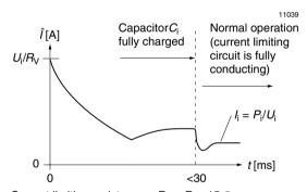
$R_V$ : Current limiting resistance =  $R_S$  +  $R_I$  = 15  $\Omega$
