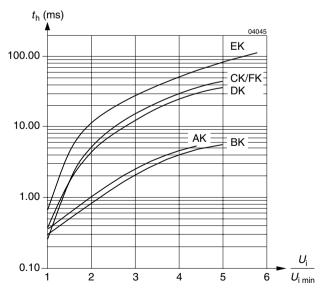
Fig. 6 Typical hold-up time  $t_h$  versus relative input voltage  $U_i/U_{i \, min}$ . The DC-DC converters require an external series diode in the input path if other loads are connected to the same input supply lines.
