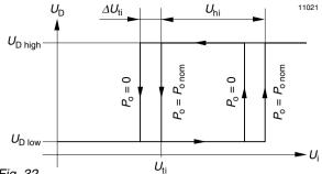
Fig. 32  $U_{ti}$  Definition of  $U_{ti}$ ,  $\Delta U_{ti}$  and  $\Delta U_{hi}$  (JFET output)
