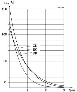
Fig. 5 Typical inrush current versus time at  $U_{i max}$ ,  $R_{ext} = 0$ . For AK, BK and FK as well as for application related values use the formula given in Inrush Current Peak Value to get realistic results.
