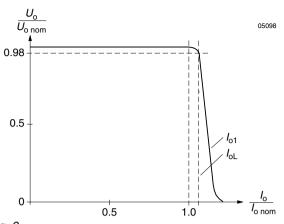
Fig. 9  $U_{01}$  vs.  $I_{01}$  (typ.) of single output units AK...EK
