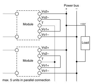
Fia. 29 Paralleling of double output units using option T with Power Bus
