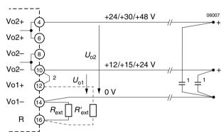
Fig. 17d AK...EK 2000 with H15 connector. R-input for output voltage control. Wiring of main and second output for two output voltages  $U_{01}$  and  $U_{02}$ : +12 V and +24 V or +15 V and +30 V or +24 V and +48 V.
