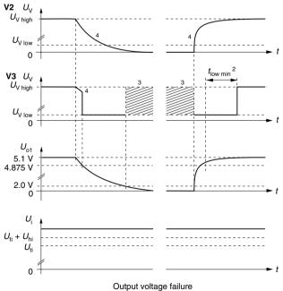
Fig. 36 Relationship between U<sub>i</sub>, U<sub>o1</sub>, U<sub>V</sub>, I<sub>V</sub> and U<sub>o1</sub>/U<sub>o nom</sub> versus time.
