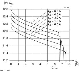
Fig. 10 AK...EK 2320:  $\Delta U_{\rm o2}$  (typ.) vs.  $I_{\rm o2}$  with different  $I_{\rm o1}$
