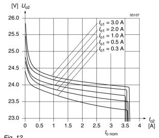
AK...EK 2660:  $\Delta U_{02}$  (typ.) vs.  $I_{02}$  with different  $I_{01}$
