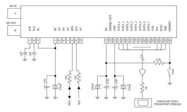
Fig 2. CONNECTION DIAGRAM
