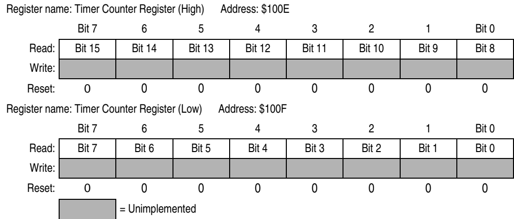
Figure 9-15. Timer Counter Register (TCNT)
