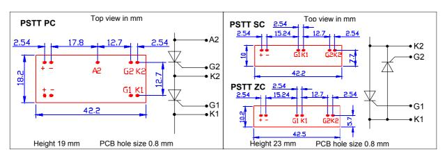
**PSTT ZC** - zero crossing switching – heating, welding, power factor correction
