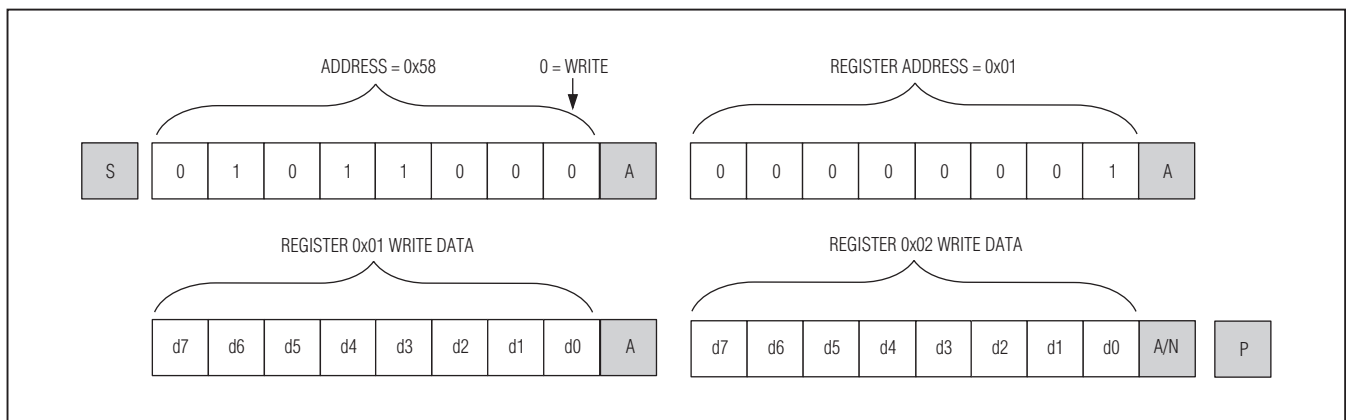
Figure 10. Format for Writing to Multiple Registers
