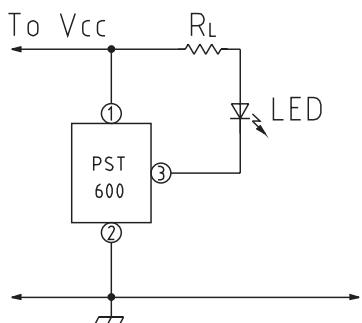
Note : When Vcc line impedance is high, connect a capacitor between IC Pins 1 and 2.
