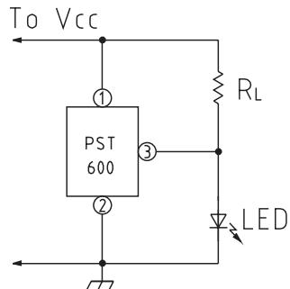
Note : When Vcc line impedance is high, connect a capacitor between IC Pins 1 and 2.
