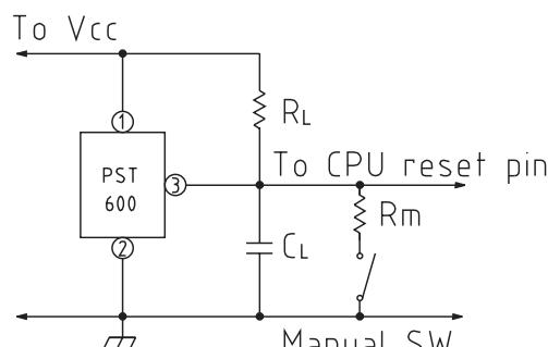
Note : Prevent Manual SW chattering by using R<sub>L</sub>, C<sub>L</sub> and R<sub>m</sub>. R<sub>m</sub> setting conditions are as follows :
