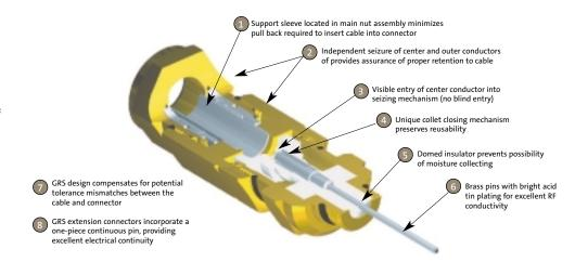
The industry leading GRS 3-piece trunk & distribution connector series are designed for optimal performance in high bandwidth, two-way and digital communication systems.
