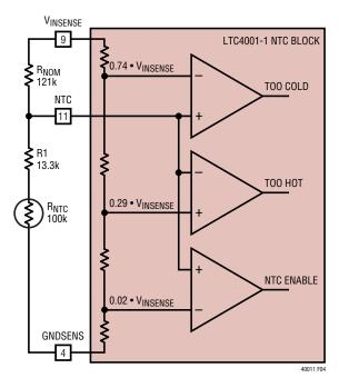
Figure 4. Extending the Delta Temperature
