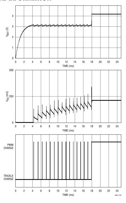
Figure 7. Battery-Less Start-Up
