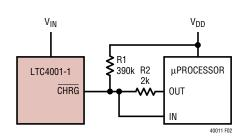
Figure 2. Microprocessor Interface
