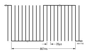
Figure 3. CHRG Temperature Fault Waveform
