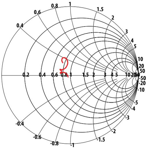
**Figure 16. Tx Port Impedance in Tx Band.**
