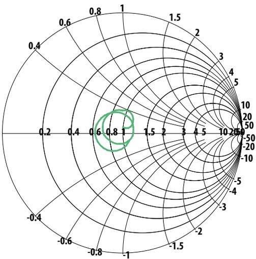
**Figure 18. Ant Port Impedance in Tx Band.**
