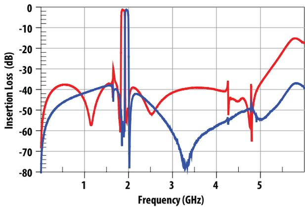
Figure 7. Tx-Ant and Ant-Rx Wideband Insertion Loss.
