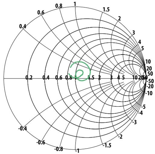
**Figure 19. Ant Port Impedance in Rx Band.**
