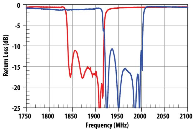
Figure 5. Tx and Rx Port Return Loss.
