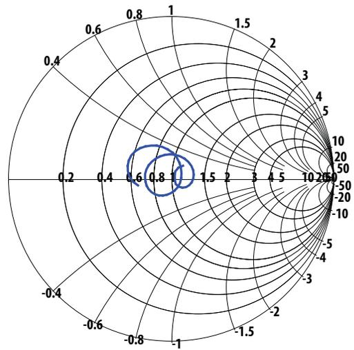
**Figure 17. Rx Port Impedance in Rx Band.**
