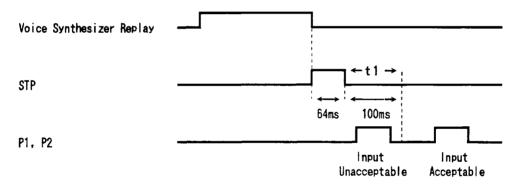
t1: The unacceptable period of input signal (about 100ms)
