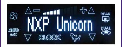
NXP display demo with COG LCD driver PCA8538 & capacitive sensor PCA8885
