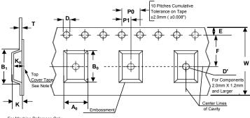
For Machine Reference Only Including Draft and RADLL Concentric Around B<sub>0</sub>
