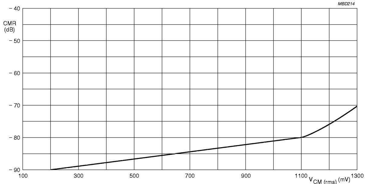
Fig.7 Common-mode rejection ratio as a function of input voltage;  $f = 1$  kHz.
