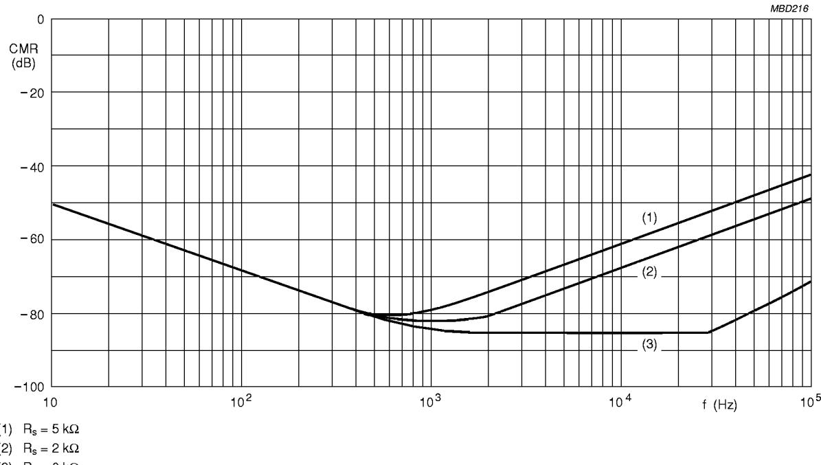
Fig.5 Common-mode rejection ratio as a function of frequency;  $V_{CM} = 1 \text{ V}$  (RMS).
