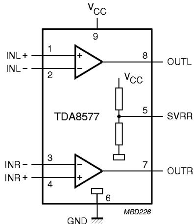
Fig.1 Block diagram.
