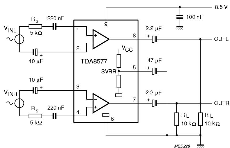
Fig.10 Application circuit with balanced signal source
