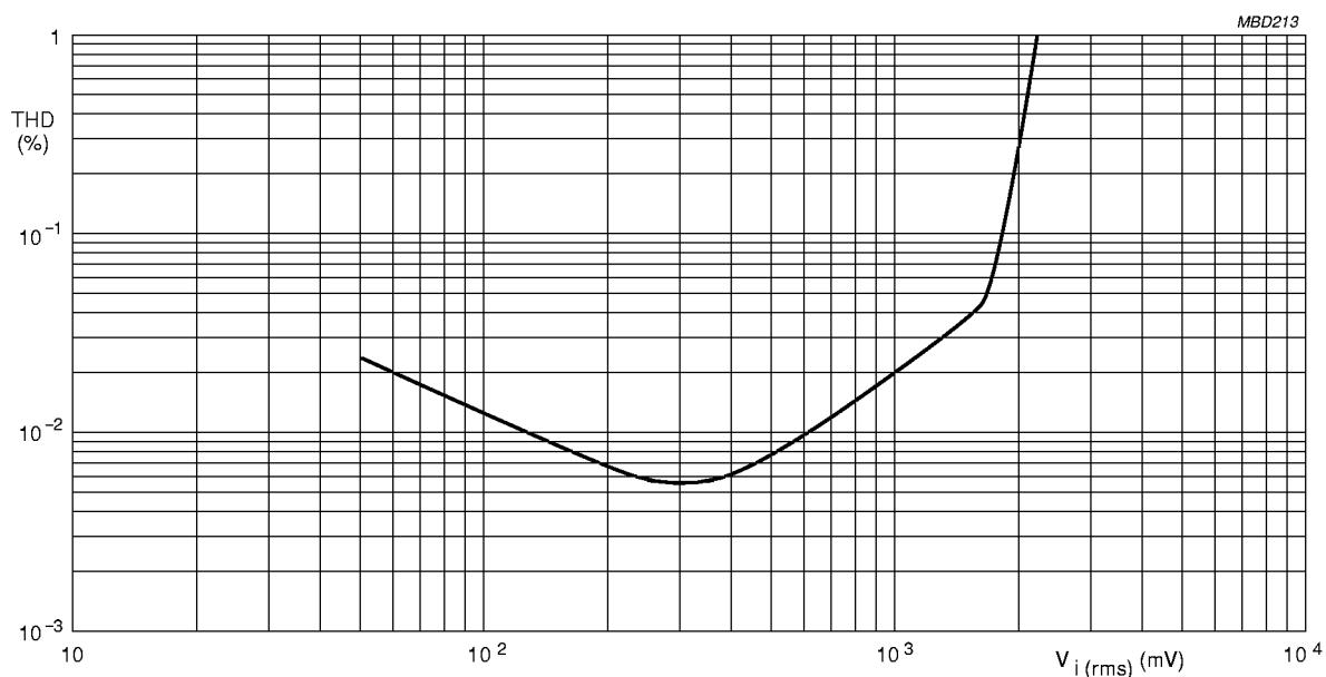
Fig.6 Total harmonic distortion as a function of input voltage;  $f = 1 \text{ kHz}$ .
