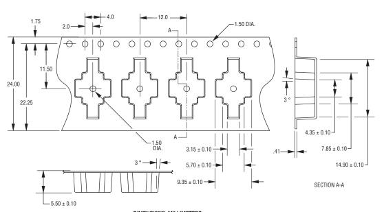
DIMENSIONS: MILLIMETERS DIMENSION TOLERANCE: .X  $\pm 0.25$
