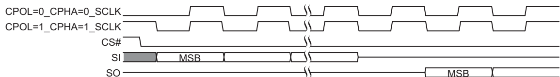
Figure 4.1 SPI Modes Supported
