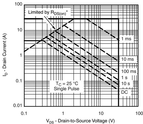
\*  $V_{DS} >$  minimum  $V_{GS}$  at which  $R_{DS(on)}$  is specified
