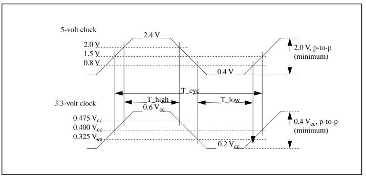
Figure 8-1 PCI Clock Waveforms
