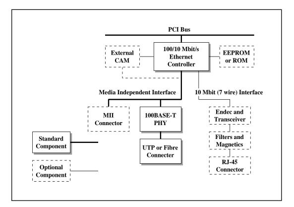
Figure 1-3 Configuration for 100BASE-T Showing Options
