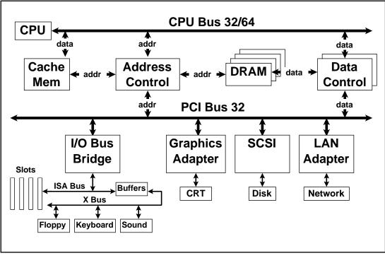
Figure 1-2 PCI System Block Diagram
