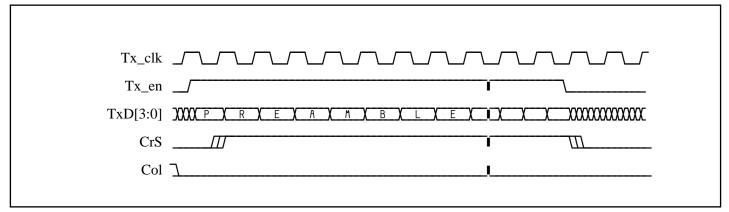
Figure 6-1 Transmission Without Collision
