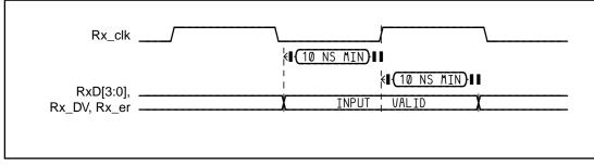
Figure 8-5 Receive signal timing relationships at the MII
