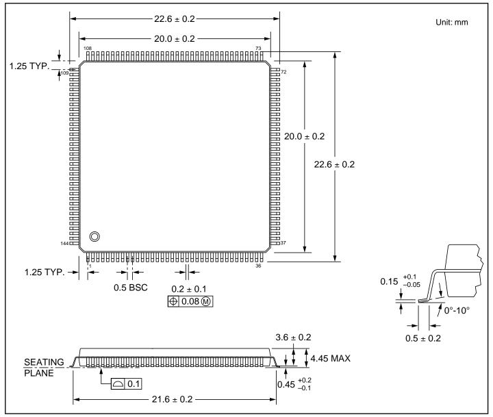
Figure 10-1 QFP144-P-2020-0.50 [144-Pin Quad Flat Package]
