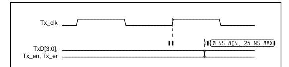
Figure 8-4 Transmit signal timing relationships at the MII
