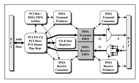
Figure 3-1 DMA Functional Blocks
