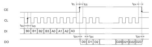
(Note) DO pin is an Nch open drain pin, so that the data varying time (tDC and tDH) differs depending on the pull-up resistance and substrate capacity.
