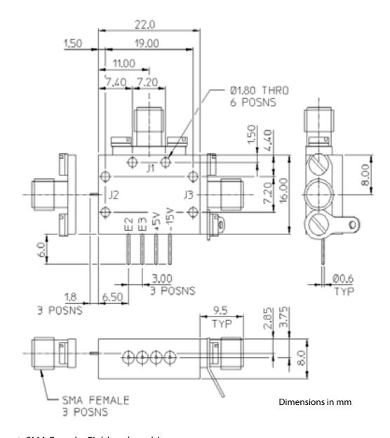
Input: SMA Female, Field replaceable
