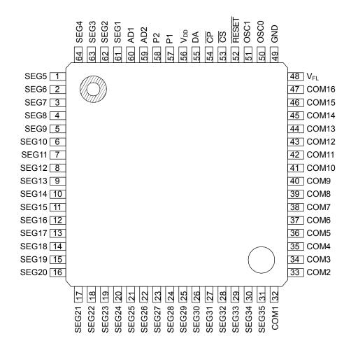
64-Pin Plastic QFP / TQFP
