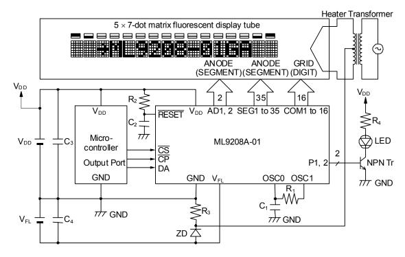
Notes: 1. The  $V_{DD}$  value depends on the power supply voltage of the microcontroller used. Adjust the values of the constants  $R_1$ ,  $R_2$ ,  $R_4$ ,  $C_1$ , and  $C_2$  to the power supply voltage used.
