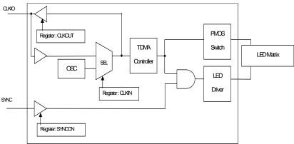
Figure 15. I/O part equivalent circuit diagram
