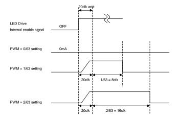
Figure 11. LED output current timing and a PWM cycle
