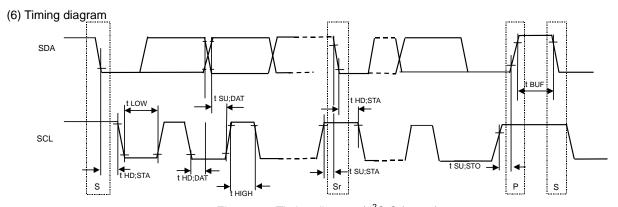
Figure 7. Timing diagram ( I<sup>2</sup>C C format)
