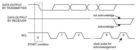
Figure 6. Acknowledge (I<sup>2</sup>C format)
