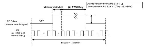
Figure 10. LED output current timing and PWM cycle
