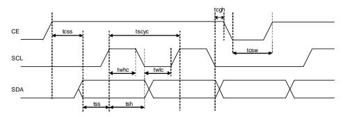
Figure 3. Timing diagram (SPI format)
