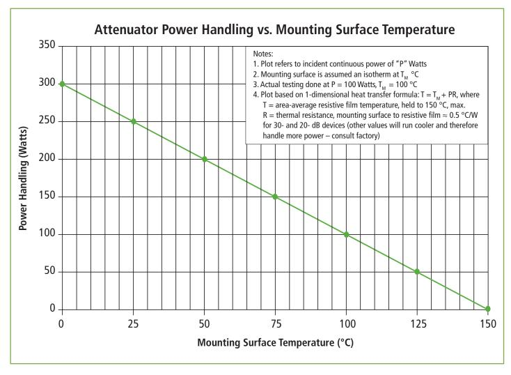
\* Test Condition: With mounting surface temperature = 75 °C, max. (see plot above). Actual test conditions are as follows: Flange attached to a large copper carrier whose surface, directly under the flange center, is held at 100 °C; power applied = 100 Watts. Specification: The attenuation shall change no more that 0.2 dB during and after a 100-hr. Burn-in per MIL-PRF-55342.
