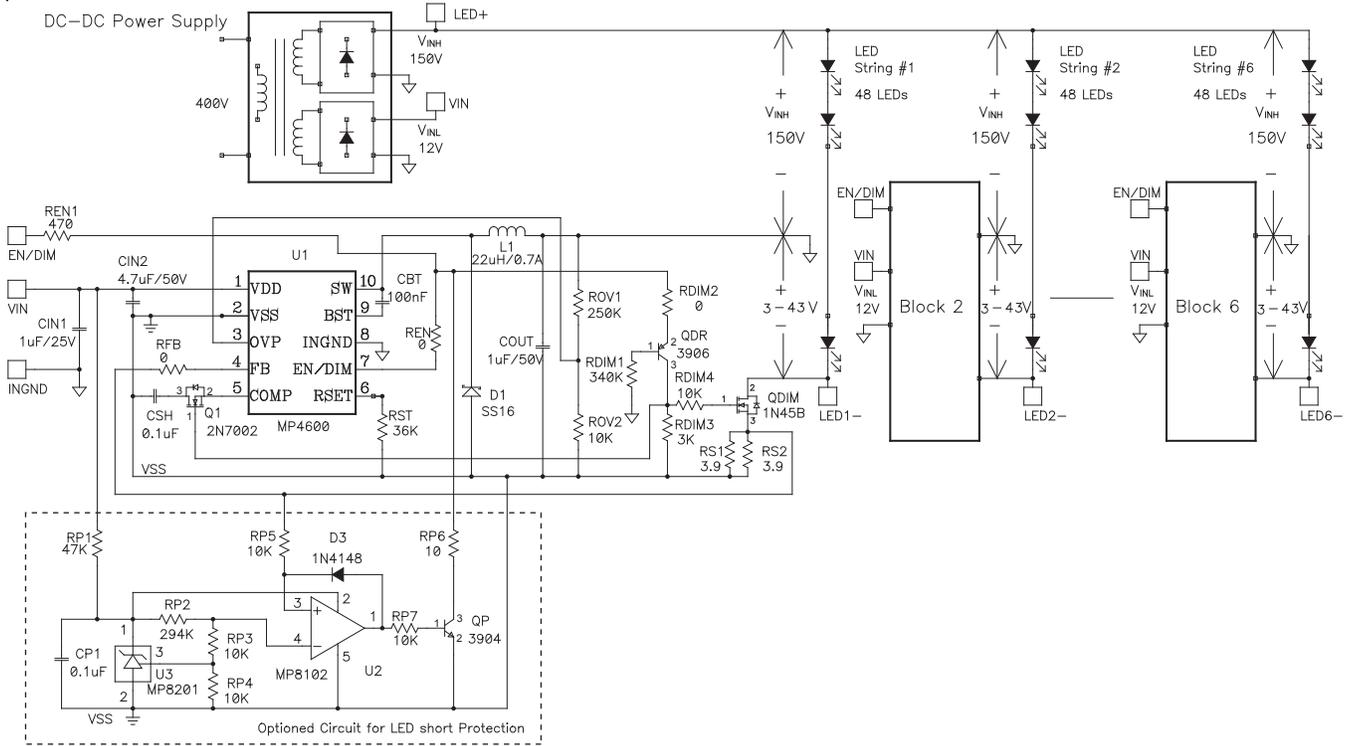
Figure 2—White LED Driver Application for TV Applications
