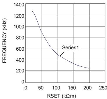
If RSET pin is floating, the setting frequency is the default value 1.35MHz.
