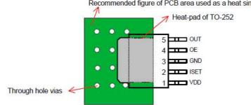
Recommended figure of PCB area used as a heat sink.
