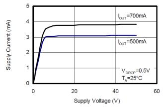
Figure 1. Supply Current vs. Supply Voltage
