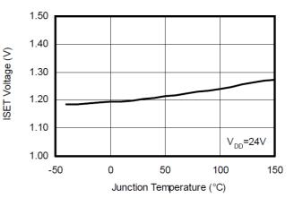
Figure 2. ISET Voltage vs. Junction Temperature
