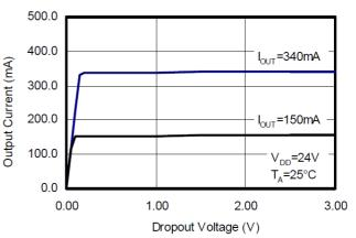
Figure 4. Output Current vs. Dropout Voltage
