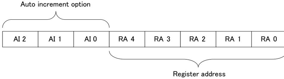
Figure 6. Register address
