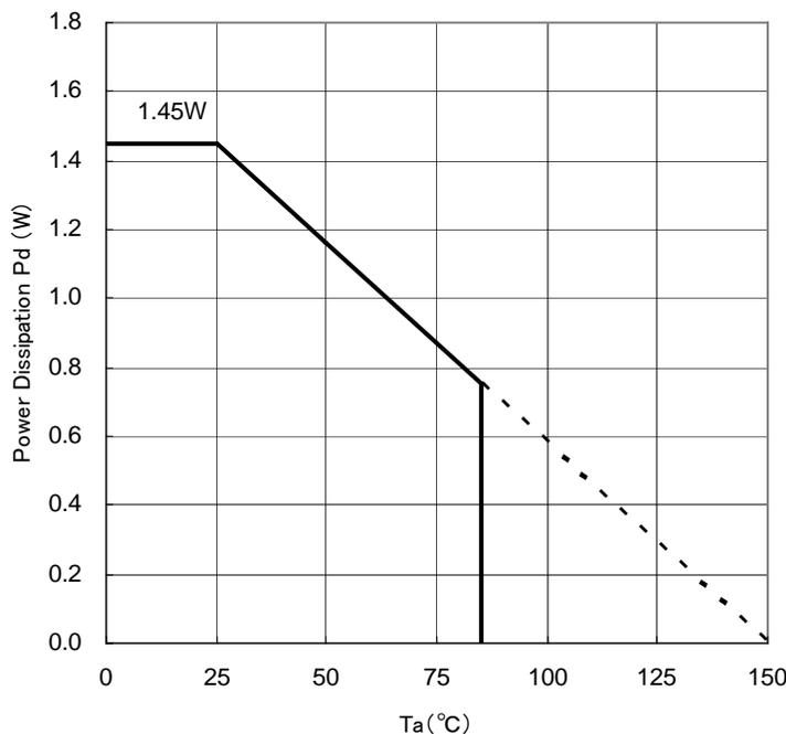
Figure 7. Power dissipation
