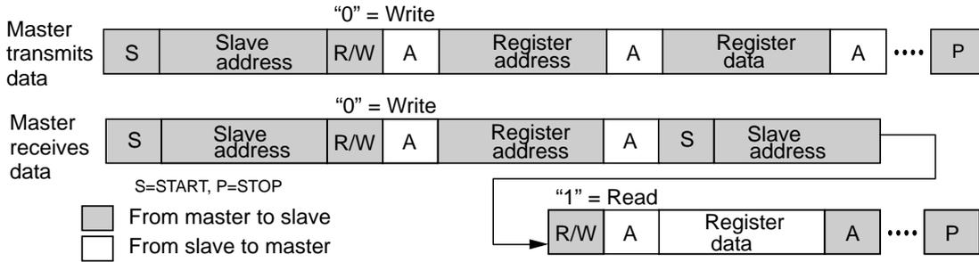
Figure 2. Basic format of control command (I<sup>2</sup>C)
