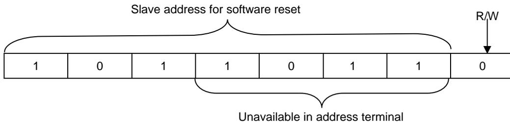
Figure 5. Slave address for software reset
