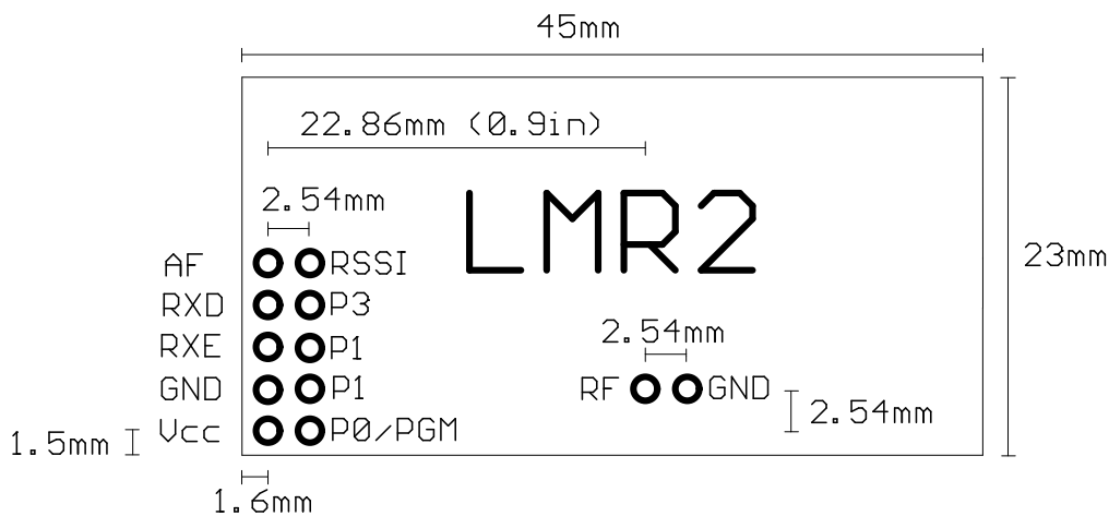
Figure 5: LMR2 footprint (top view)
