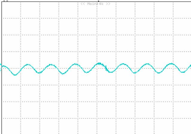
**Figure 5: Output Ripple & Noise**
