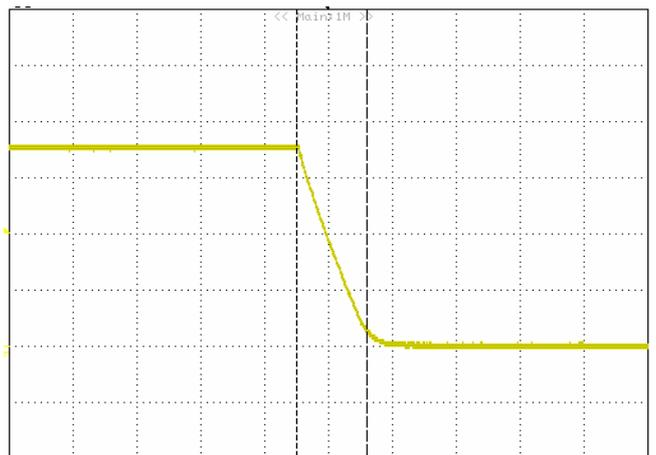
**Figure 10:** Output Fall Time: 1 pcs Converter on test board.
