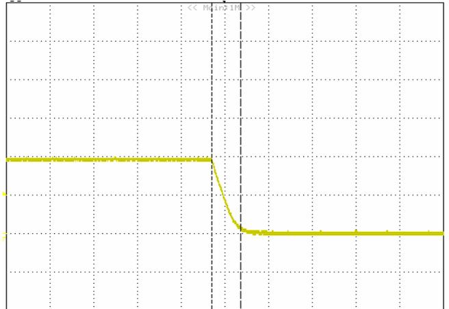
**Figure 8:** Output Fall Time: 1 pcs Converter on test board.
