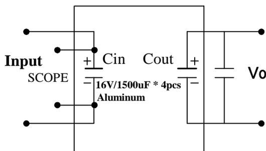
**Figure 13:** Peak-peak Input ripple & noise measurement test setup
