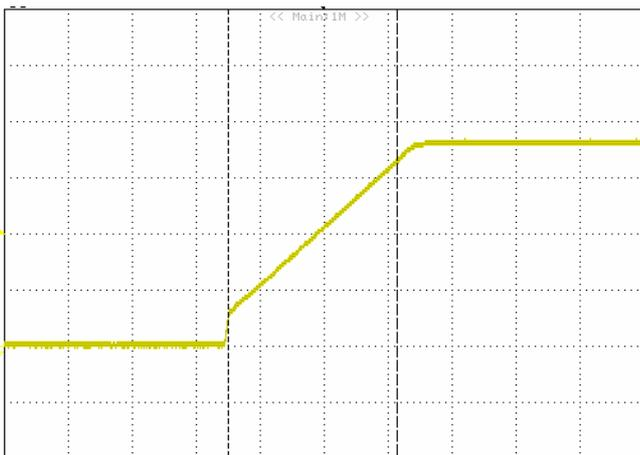
**Figure 9:** Output Rise Time: 1 pcs Converter on test board.
