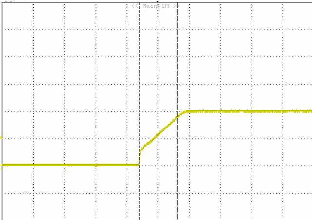
**Figure 7:** Output Rise Time: 1 pcs Converter on test board.
