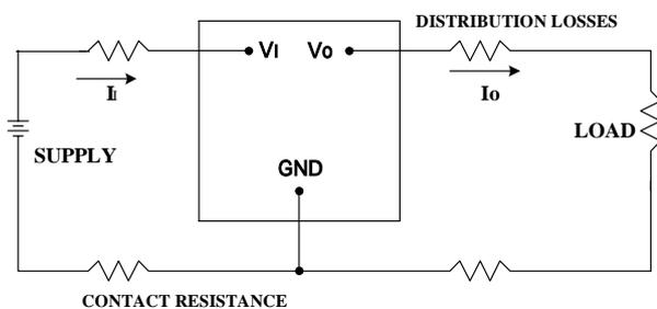
**Figure 12:** Output voltage and efficiency measurement test setup
