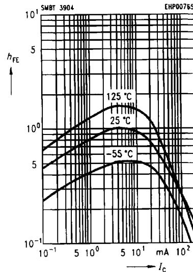
**Short-circuit forward current transfer ratio**
