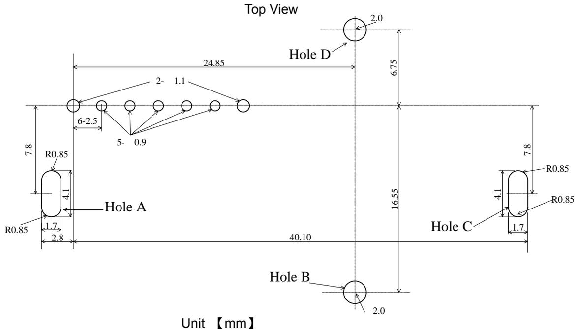
Metal case is connected to GND. So hole A,B,C and D should be connected to GND.
