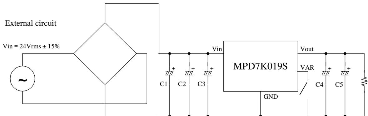
C1,C2,C3 : 1000μF/50V Low Impedance Aluminum Electrolytic Capacitor (EKZE500EC3102ML25S NIPPON CHEMI-CON)
