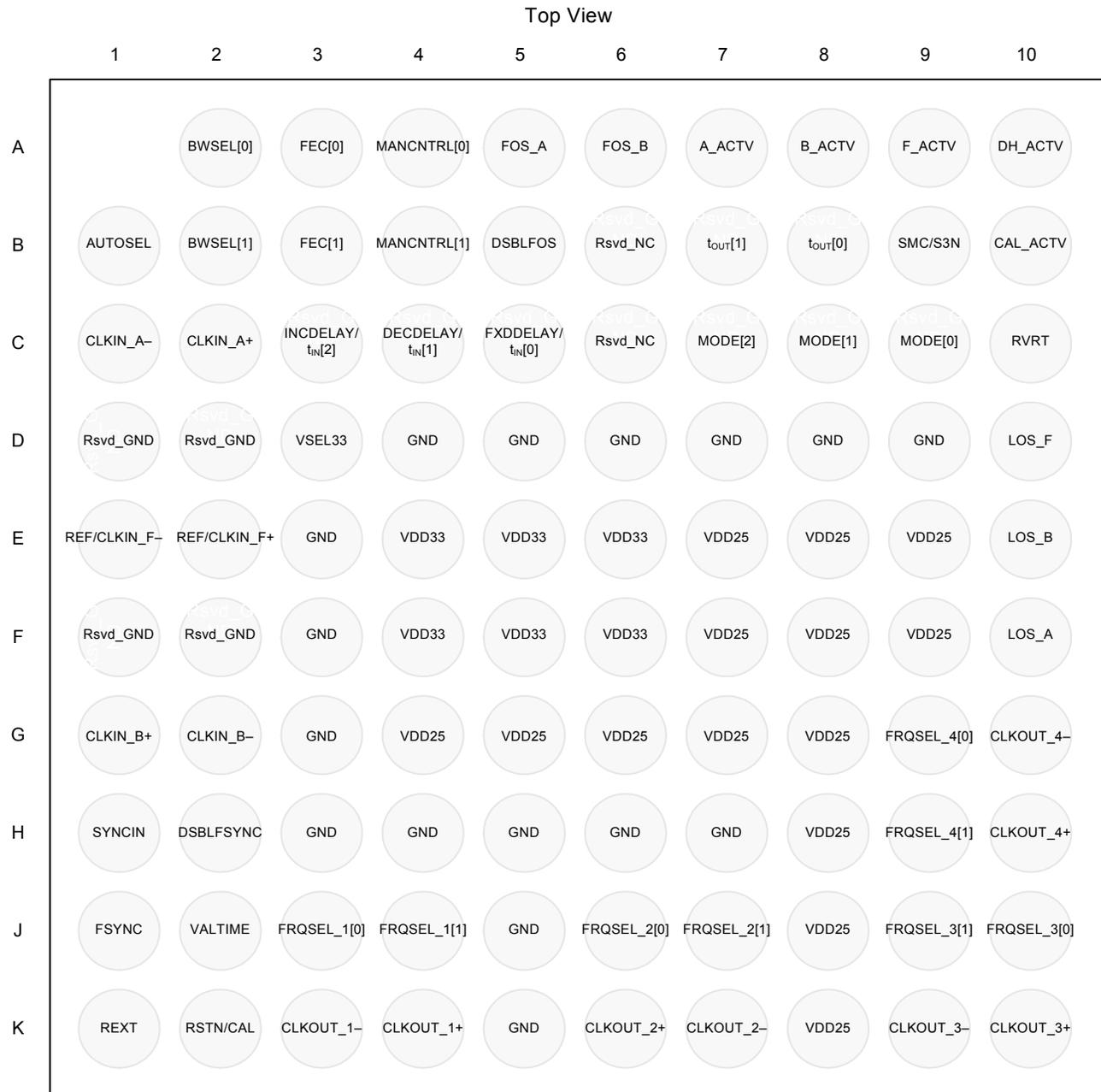
**Figure 16. Si5364 Pin Configuration (Transparent Top View)**
