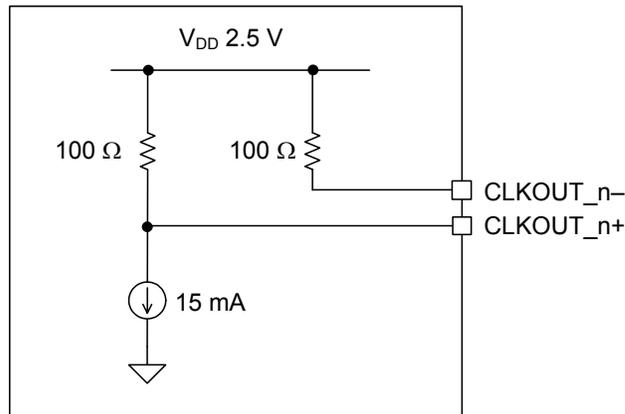
Figure 13. CLKOUT\_n± Equivalent Circuit, RSTN/CAL asserted LOW
