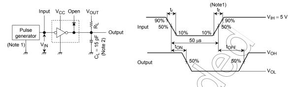
Note 1: Pulse width 50  $\mu$ s, duty cycle 10%, output impedance 50  $\Omega$ ,  $t_f \le 5$  ns,  $t_f \le 10$  ns
