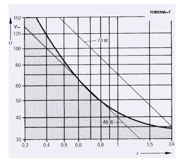
d = switching currentU = switching voltage
