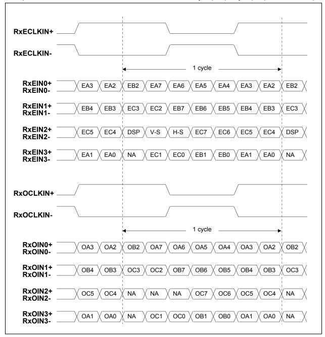
Note: A/B/C data 7: MSB, A/B/C data 0: LSB, DSP = DSPTMG, V-S = Vsync, H-S = Hsync, x: A (Stripe A)or B(Stripe B)
