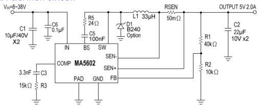
$V_{OUT}$ = $V_{FB}$  × (1+R1/R2),  $V_{FB}$  = 1.00V, R2 suggest 10k~30KΩ  $I_{SEN}$  =  $V_{SET}$  / RSEN-  $\triangle$  I/2  $\rightleftharpoons$  120mV / 50mΩ-0.2A = 2.2A
