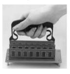
Insert the jig protrusion in the board hole. Grasping the handle, pull the board up.
