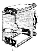
MONOJACKS ARE CAPTIVATED IN KEYHOLE SLOT OF HOOD AS SHOWN ABOVE. WHEN USING SHELLS, MONOJACKS ARE CAPTIVATED IN KEYHOLE OF SHELL AND CLEARANCE HOLES ARE PLACED IN HOODS.
