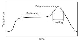
For soldering (Example: Sn/Pb)
