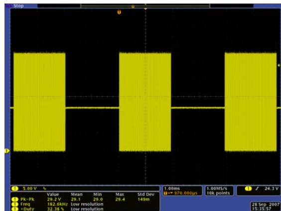
FIGURE 13. LX AT 50% PWM DIMMING (54 LEDs, 20mA, V IN = 12V)
