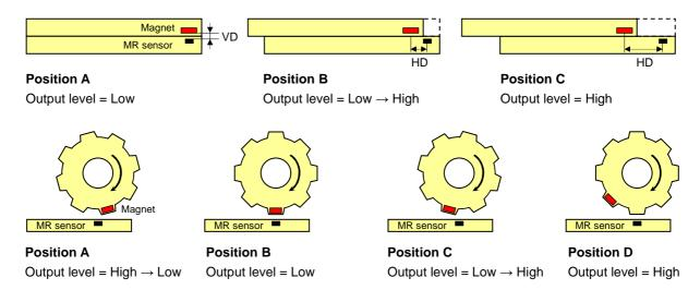
In the detection of the slide type, there are two ways of arrangement of magnetic field detecting direction against moving direction. One is parallel and another is cross with moving direction.
