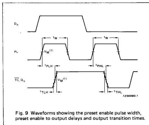
Fig. 9 Waveforms showing the preset enable pulse width, preset enable to output delays and output transition times.
