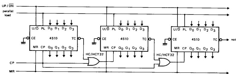
Fig. 13 Cascading counter packages (ripple clocking).
