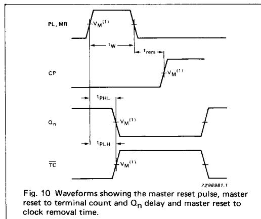
Fig. 10 Waveforms showing the master reset pulse, master reset to terminal count and  $Q_n$  delay and master reset to clock removal time.
