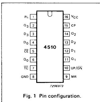
Fig. 1 Pin configuration.
