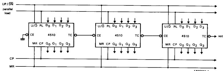
Fig. 12 Cascading counter packages (parallel clocking).
