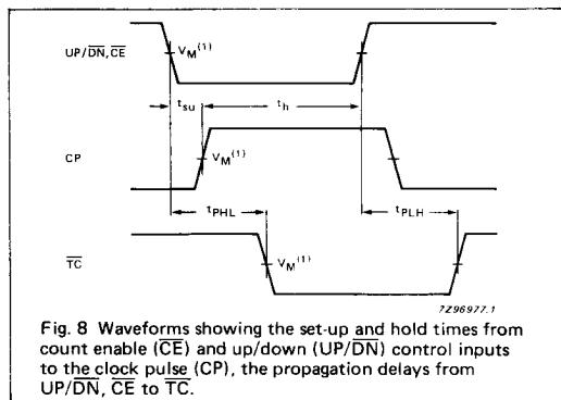
Fig. 8 Waveforms showing the set-up and hold times from count enable (CE) and up/down (UP/DN) control inputs to the clock pulse (CP), the propagation delays from UP/DN, CE to  $\overline{TC}$ .
