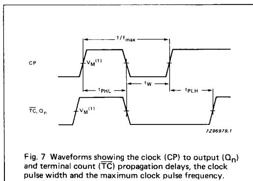
Fig. 7 Waveforms showing the clock (CP) to output ( $Q_n$ ) and terminal count ( $\overline{TC}$ ) propagation delays, the clock pulse width and the maximum clock pulse frequency.
