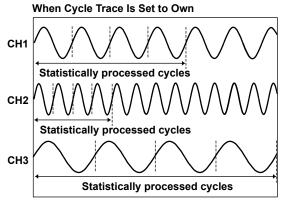
The number of cycles in the channel with the slowest cycle (CH3) is four, so statistical processing is performed on the four oldest cycles of the data for CH1 and CH2. The remaining data is not used for statistical processing.
