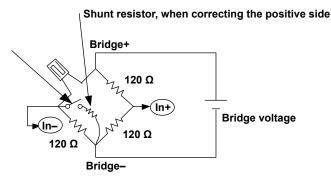
On the DL850/DL850V, in addition to performing normal shunt calibration (when the shunt-calibration relay circuit is on), you can also set the zero-point value when the relay circuit is off. The zero-point value is valid when the strain value after balancing is performed is not 0.
