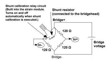
· When correcting the gain on the positive side
