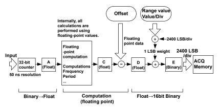
The frequency module measures the period of the input signal using a 32-bit counter at a resolution of 50 ns. Therefore, the minimum resolution of the counter values is 50 ns.
